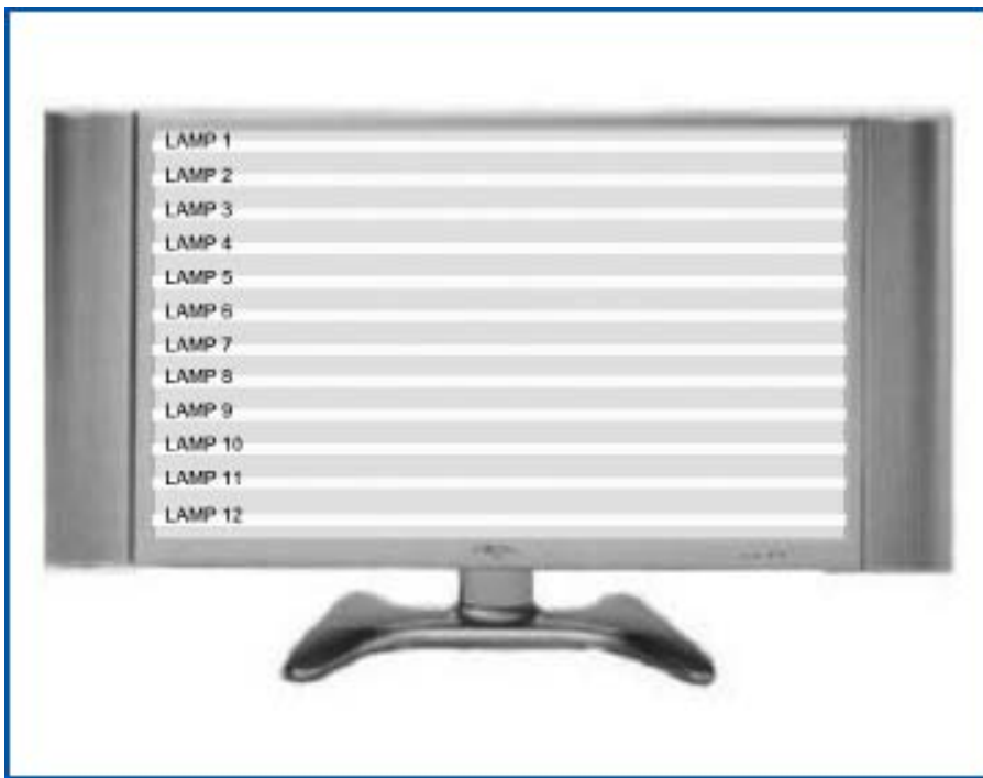
Figure 12. LCD TVs contain from 4 to 40 CCFLs.
